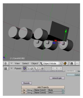
Figure 2 - A constrain between the rover's main body and a wheel. Notice the properties (box on the bottom) that define the parameters.
